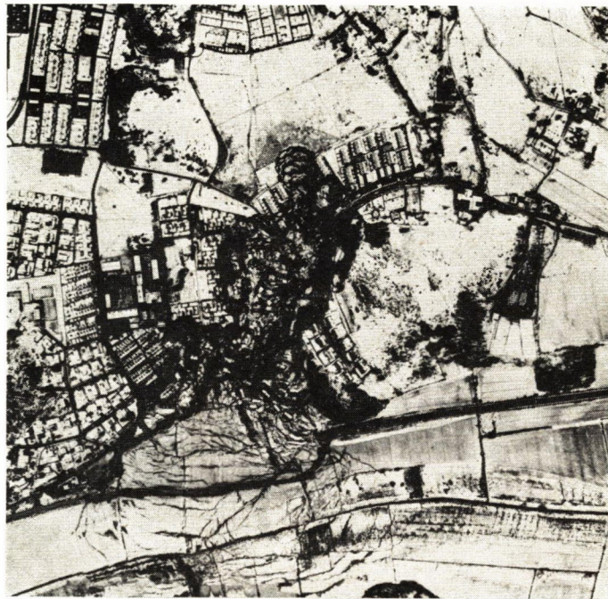
Fig. 1. The landslide in Tuve covered an area of 27 ha. In the upper "active" zone of the slide, the original ground surface sank a maximum of 10m. In the lower "passive" zone, the original soil was pressed upwards a maximum of 5m due to the energy of motion of the sliding soil masses. The volume of soil involved in the slide can be estimated at 3-4 million m^3 .
